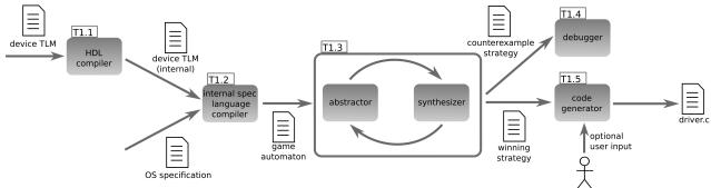
Figure 2: Architecture of the sequential driver synthesis tool.
