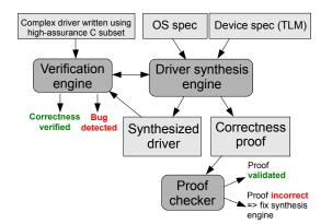
Figure 1: Overview of the driver synthesis methodology.
