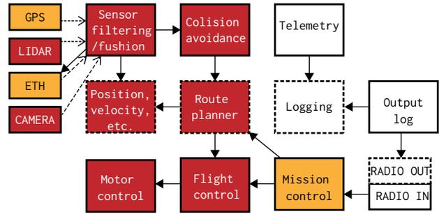
Figure 2: Simplified AAV design, showing main components (seL4 address spaces). Solid frames indicate active components, broken frames passive ones. Solid arrows indicate RPC-style server invocation, dashed arrows are completion signals. For clarity we do not show most invocations of the logging service, this would add a solid arrow from each component to the “Logging” box. Most critical components are shown in red, least-critical ones in white.
