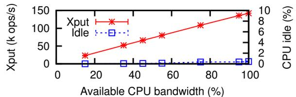
Figure 10: Throughput of Redis YCSB workload A and idle time vs available bandwidth.
