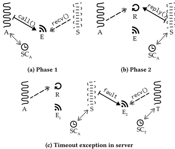
Figure 7: IPC between an active client and passive server: (a) shows the initial rendezvous, (b) shows the reply.  $SC_A$  is donated between client and server. (c)  $SC_A$  expires and a fault is sent to the server’s timeout exception endpoint  $E_2$ . See Figure 6 for the symbols used.
