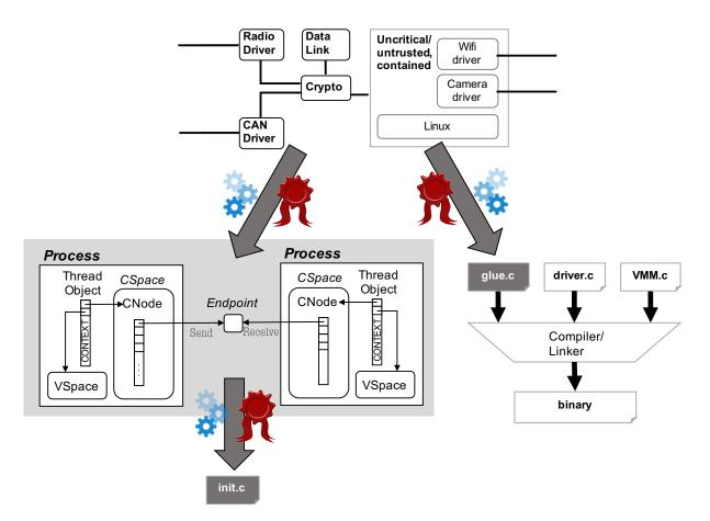
Fig. 1. Architecture enforcement. Parts in gray are generated with assurance.
