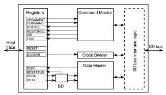
Figure 9: The OpenCores SD host controller device architecture.
