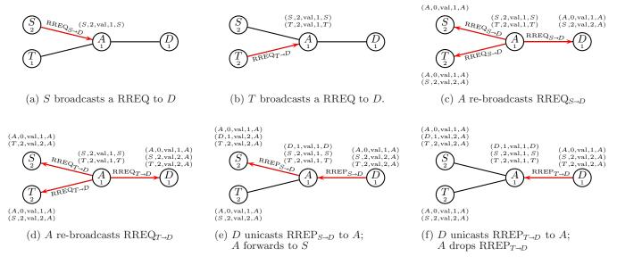
Figure 3: Failure of route discovery process
