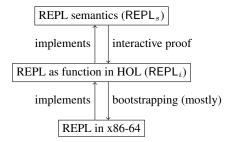
At the top is the semantic specification of the REPL. At the bottom is machine code implementing the REPL. In between is an implementation of the REPL as a function in logic. We describe the components of each layer in more detail below, then give an overview of the proof that each layer implements the one above it.
