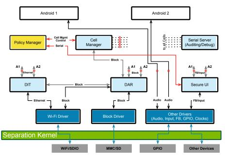
Figure 1: An example multi-persona Android platform built leveraging a separation kernel (OKL4 Microvisor) for componentization. This approach enables stronger policy controls, non-by-passable guaranteed invocation of encryption, and other high-assurance capabilities.
