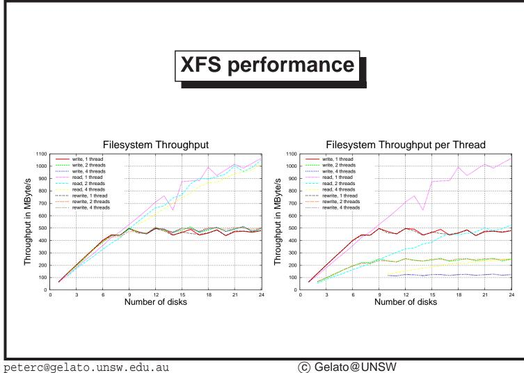
These graphs show IOZONE results XFS and Ext3, using the deadline scheduler and a 64k linux page size. The setup uses three 3ware controllers and up to 12 disks on each channel, in a RAID0 configuration.
