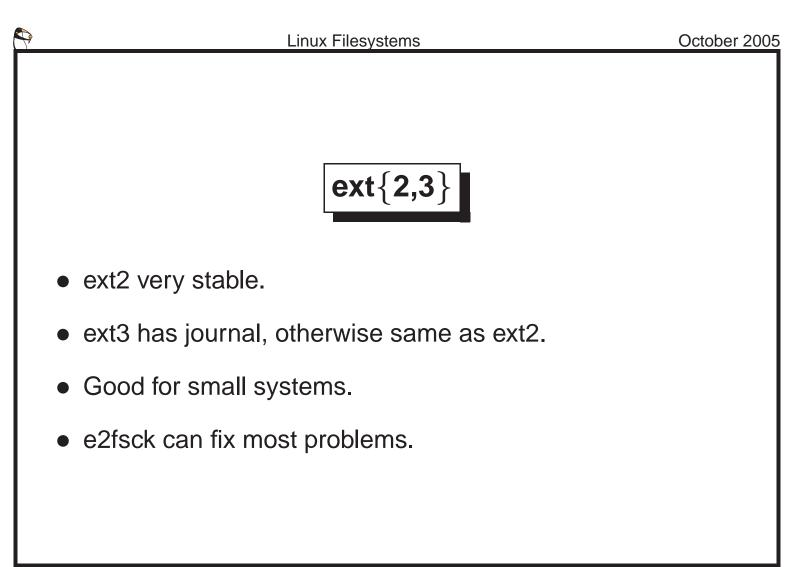
The really nice thing about ext2 is that its performance is good (at least for small numbers of spindles) and that fsck can fix almost all errors. It has a reputation for being a very robust and full-featured filesystem.
