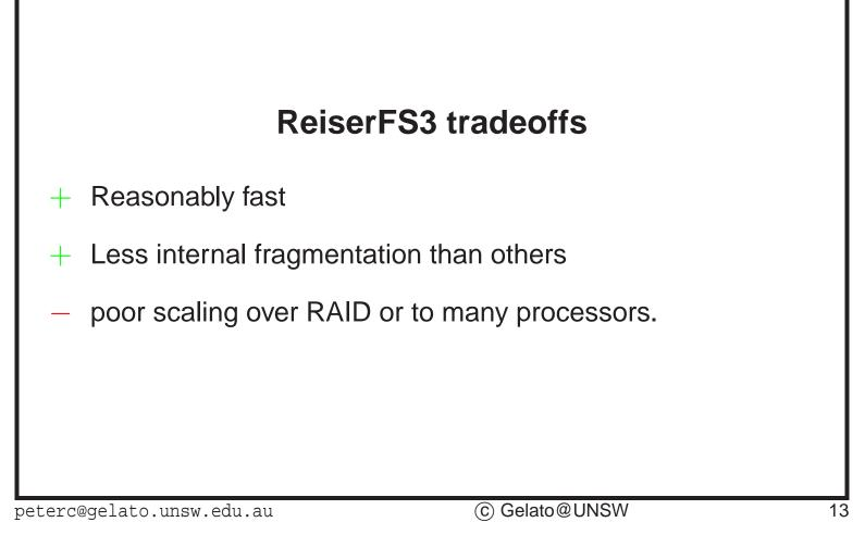
On testing ReiserFS version 3 we found it scaled neither to large numbers of processors nor large numbers of spindles in RAID.
