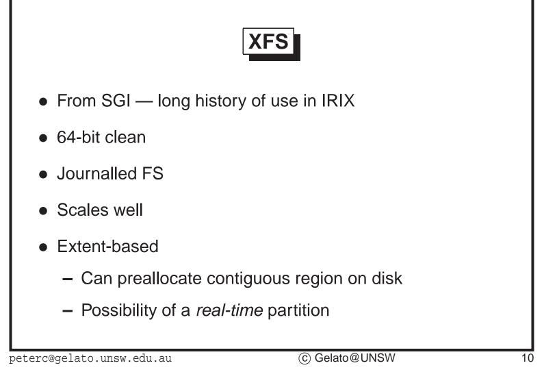
XFS is newer to Linux, but is a mature filesystem introduced first in Irix 6. It was designed to replace SGI's EFS (extent-based filesystem), removing EFS's limitations while maintaining the good performance and scalability.
