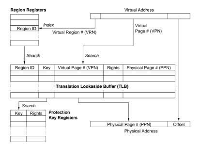
Figure 2: Itanium address translation and memory protection.
