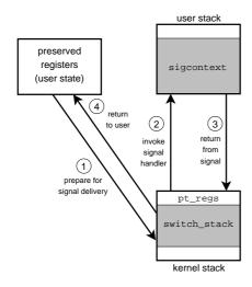
Figure 4: Steps taken during signal delivery
