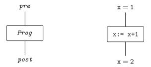
At left is a "generic" Floyd annotation of a flowchart containing only one program element. If the annotation <code>pre</code> holds "on the way in" to the program <code>Prog</code>, then annotation <code>post</code> will hold on the way out. At right is an example with specific annotations and a specific program.
