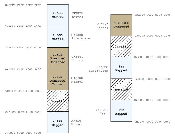
Figure 4.1: Address-space layout on the MIPS R4700.
