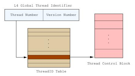
Figure 3.2: Indirectly addressing thread control blocks.
