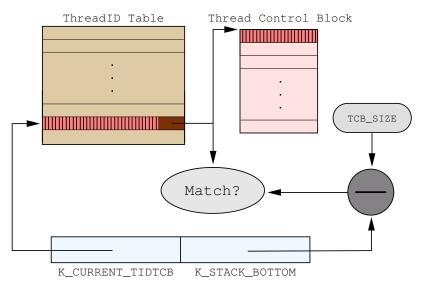
Figure 4.9: Determining if the current thread's threadID-table entry is still present in the threadID-table cache.
