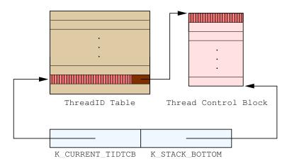
Figure 4.8: Locating the current thread's threadID-table entry on the MIPS64.
