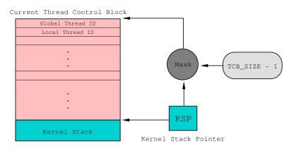
Figure 3.6: Locating the current thread's thread control block.
