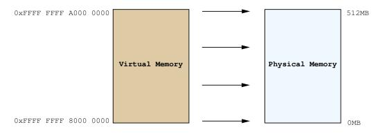
Figure 3.3: Physical addressing on the MIPS R4700.
