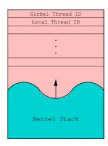
Figure 2.5: Per-thread kernel stacks in L4 reside in each thread's TCB.
