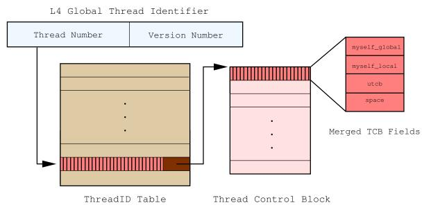
Figure 4.7: A threadID table where each entry duplicates a subset of TCB fields.
