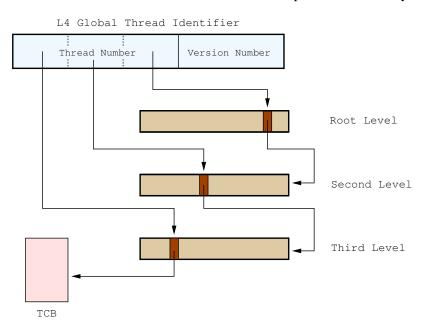
Figure 4.6: A hierarchial-table data structure for the threadID table.
