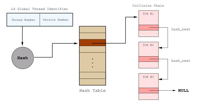
Figure 4.5: A hash-table data structure for the threadID table.
