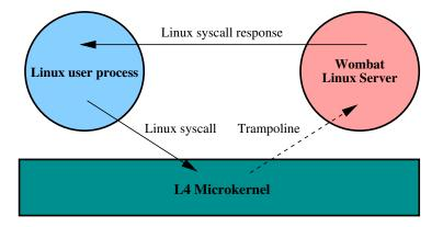
Figure 5.2: Linux system-call convention implemented via trampoline.
