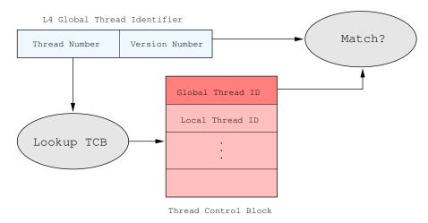
Figure 3.4: Validating thread identifiers in L4.
