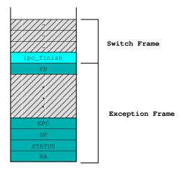
Figure 4.2: Exception and switch frames on the MIPS64 IPC-fastpath kernel stack.
