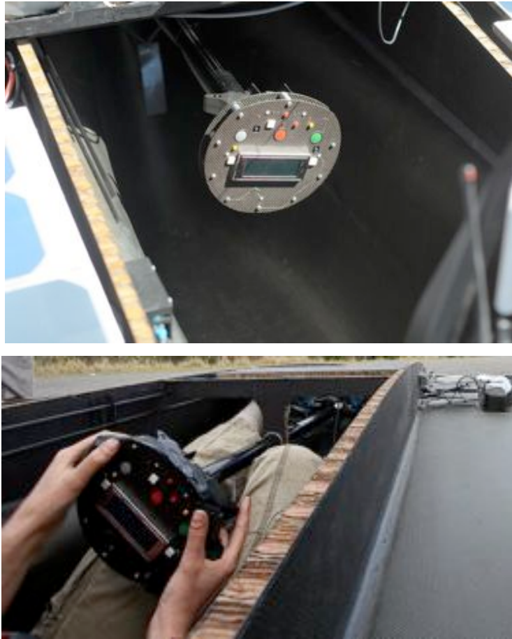
Figure 5.12: Photograph of completed version 1 steering wheel mounted in Sunswift IV. ( Top photo courtesy Matt Cumming [18], bottom photo courtesy Cameron.G.Cooke. )
