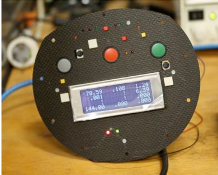
Figure 5.11: Photograph of steering cover mounted onto electronics. ( Photo courtesy Cameron.G.Cooke. )
