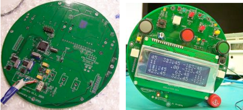
Figure 5.4: The MSP430 based, version 1 driver controls PCB developed throughout the thesis.
