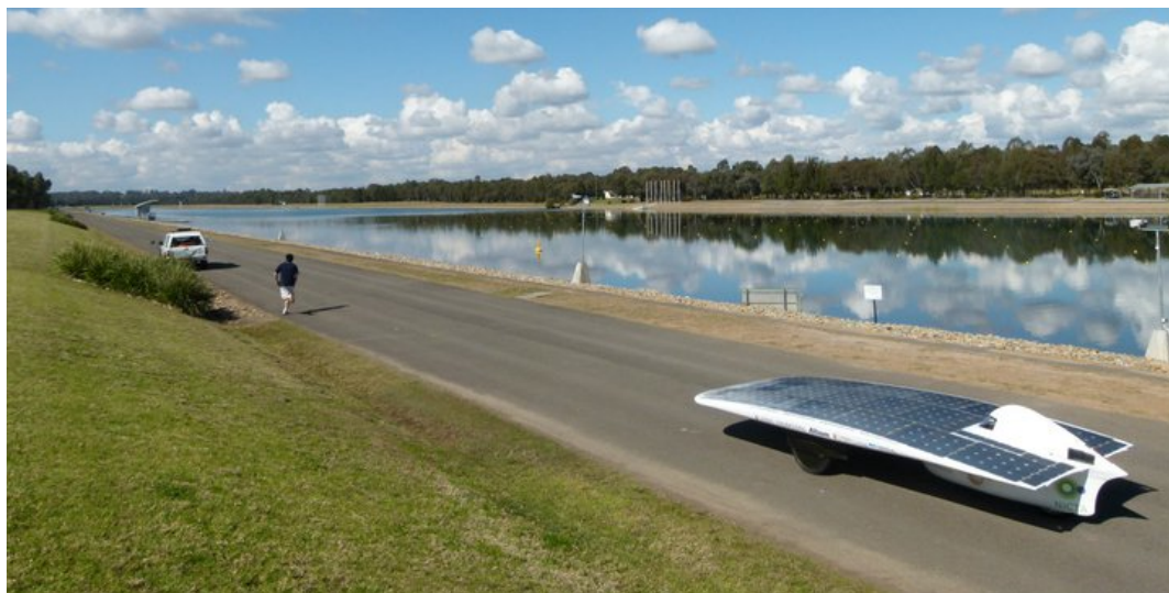
Figure 3.1: Roll-down testing Sunswift IV at the Sydney International Regatta Centre
